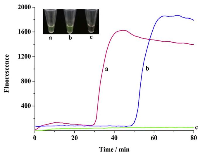
Fig. 3. Detection of different concentrations of *L. monocytogenes* total RNA by SEA method. Inset represented the corresponding colorimetric result for the amplification. a–c respectively represented the RNA concentration were 10 ng/μL, 1 ng/μL and 0 ng/μL.
